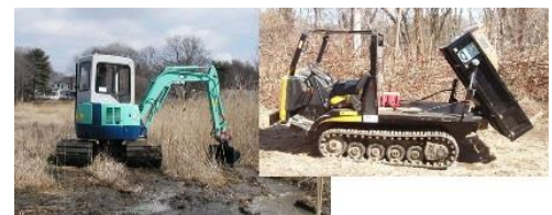
Low Ground Pressure Excavator, Mower, and Dumper for Saltmarsh water management projects.
