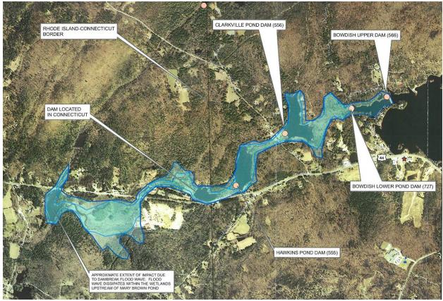
Dam failure inundation map for Bowdish Dam (No. 566), Glocester. A map specific to each dam is included in the EAP for that dam.
