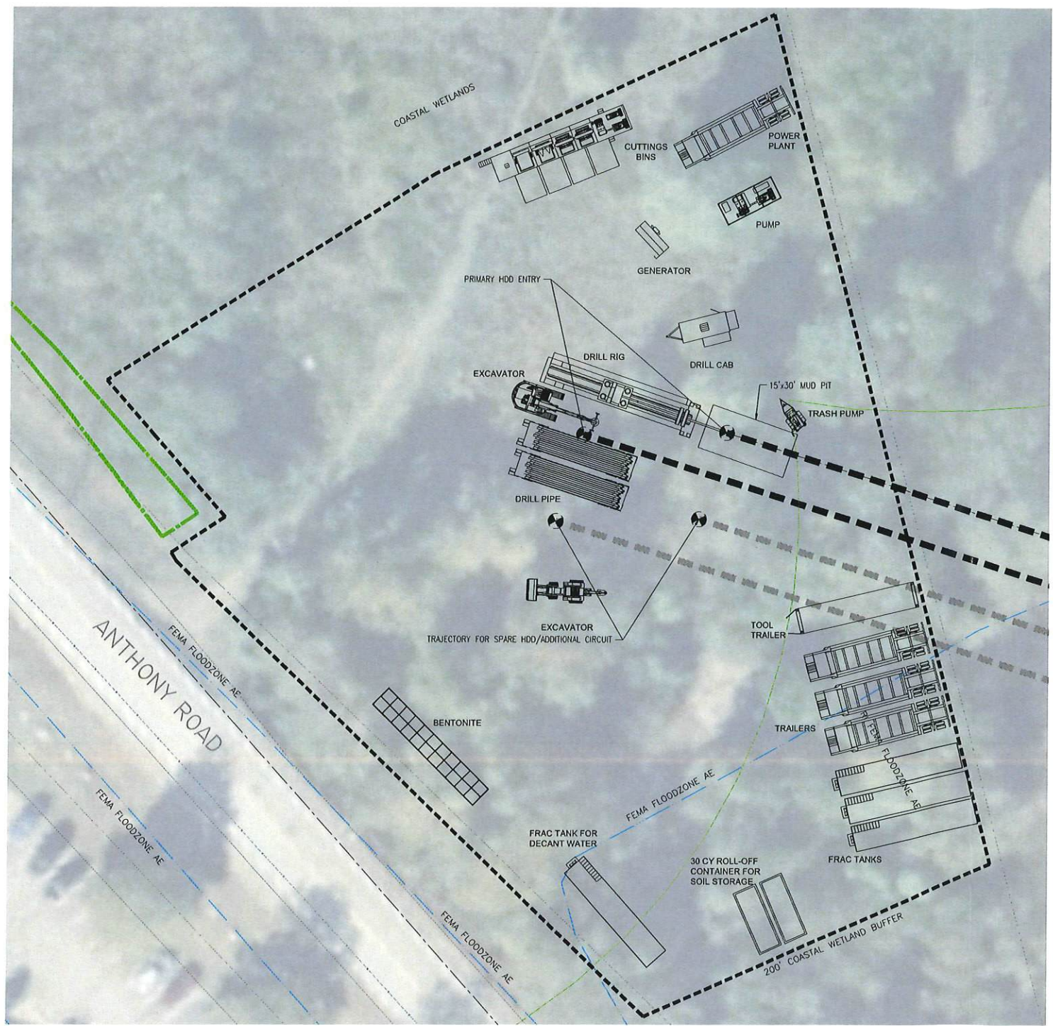
ONSHORE HDD SETUP (TYP)
