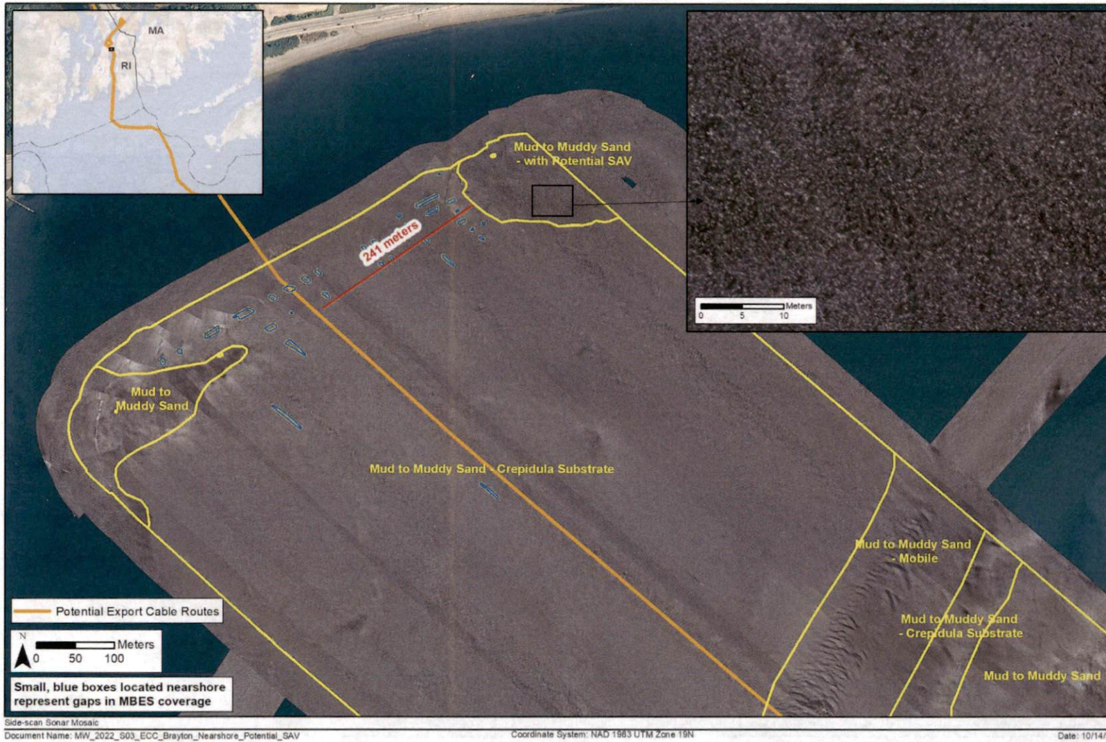
Figure 4-4. Likely presence of SAV mapped based on distinct side-scan sonar data at the east edge of the cable corridor south of Aquidneck Island
