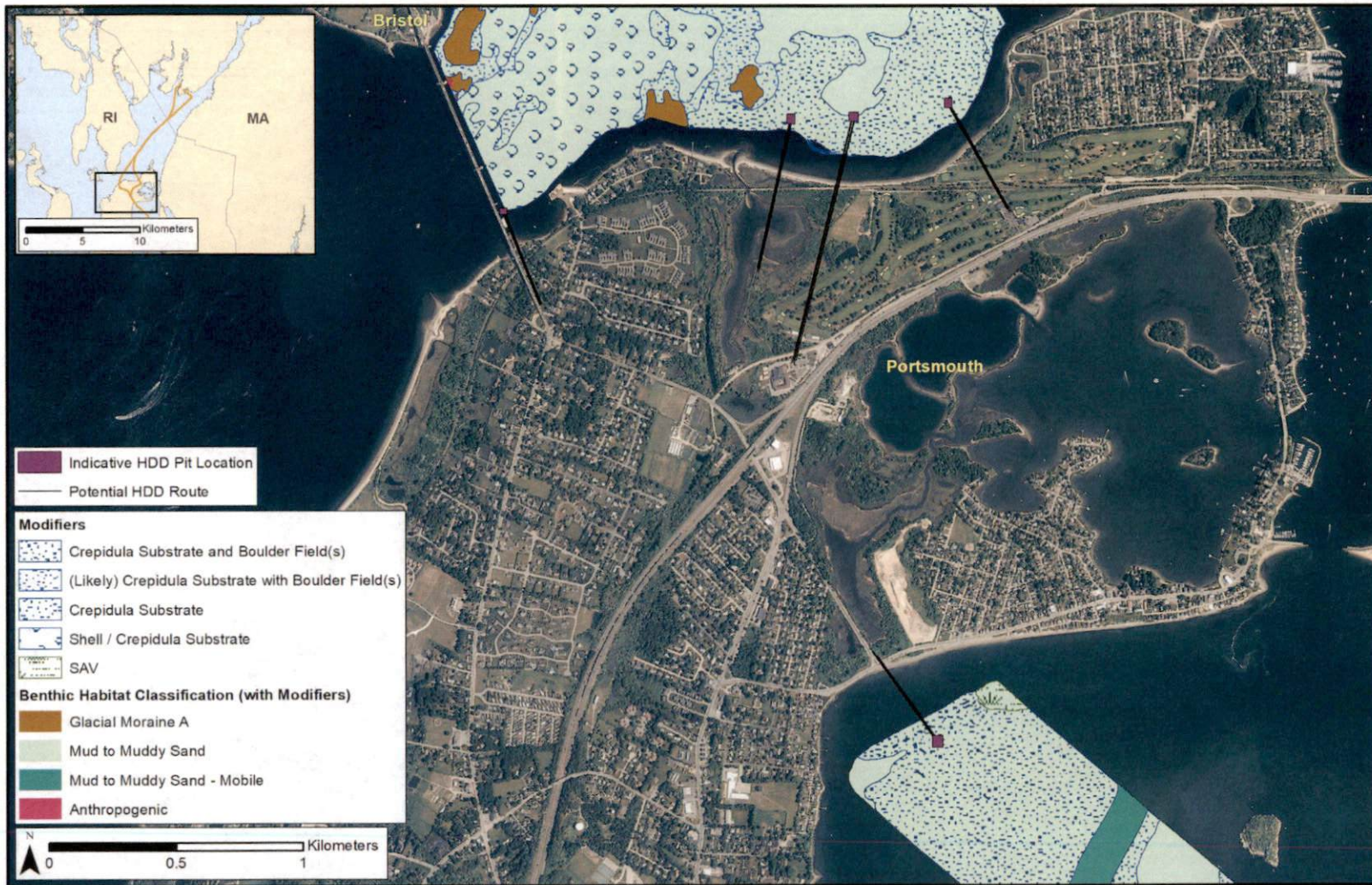
Figure 4-2. Export cable corridor and four optional locations for four HDD pits on both sides of Aquidneck Island along with benthic habitat types with modifiers
