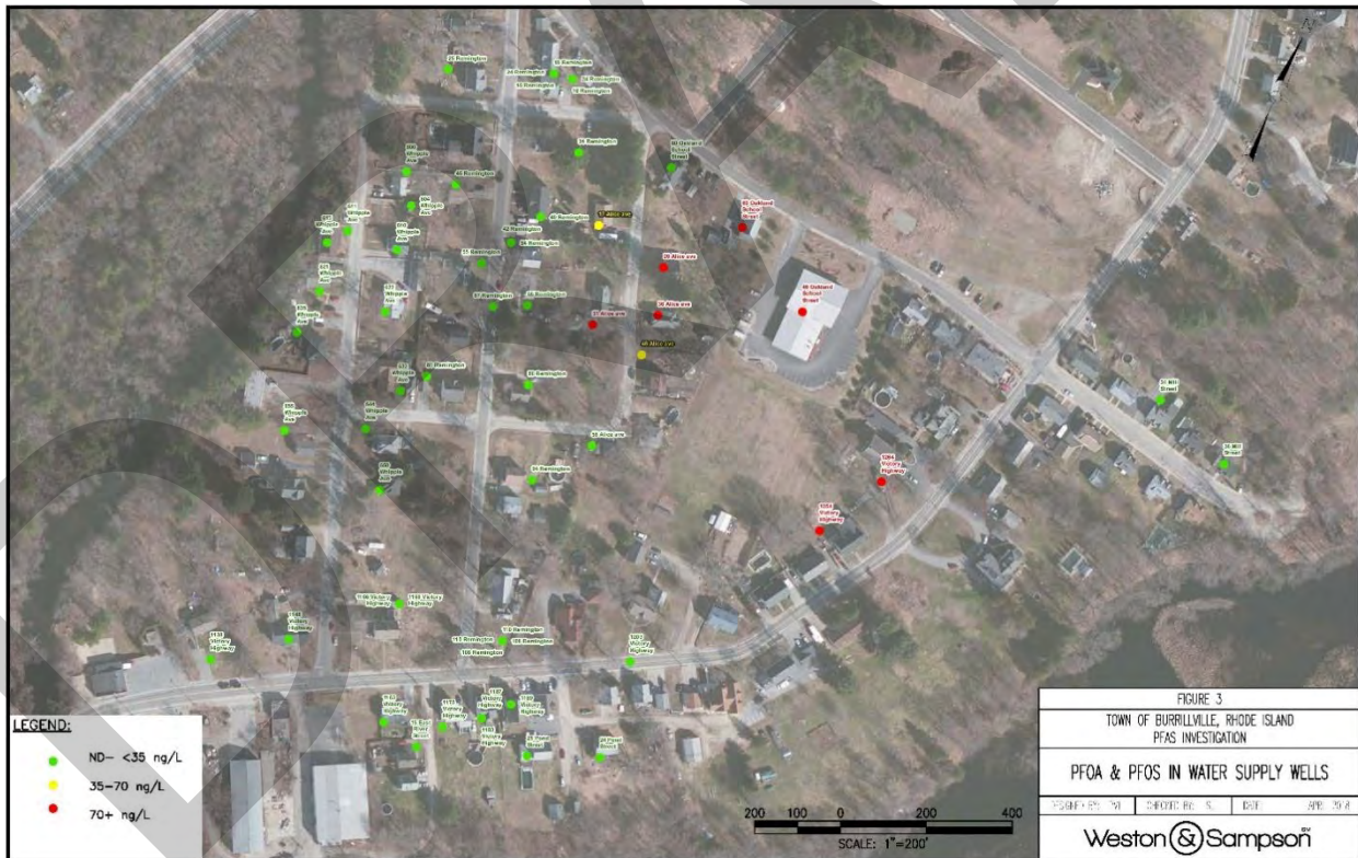
Figure 4: Map showing the results of the private well sampling in Oakland. Note the Oakland-Mapleville Fire Department is the large building in the center of the map (Weston & Sampson, 2018).
