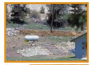
Figure 18: Keep firewood, propane tanks and natural gas meters at least 30 feet away from structures.
