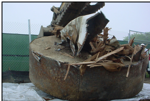
(Above) — One of two Springfield gas machine generators unearthed during the redevelopment of the Ocean House.
