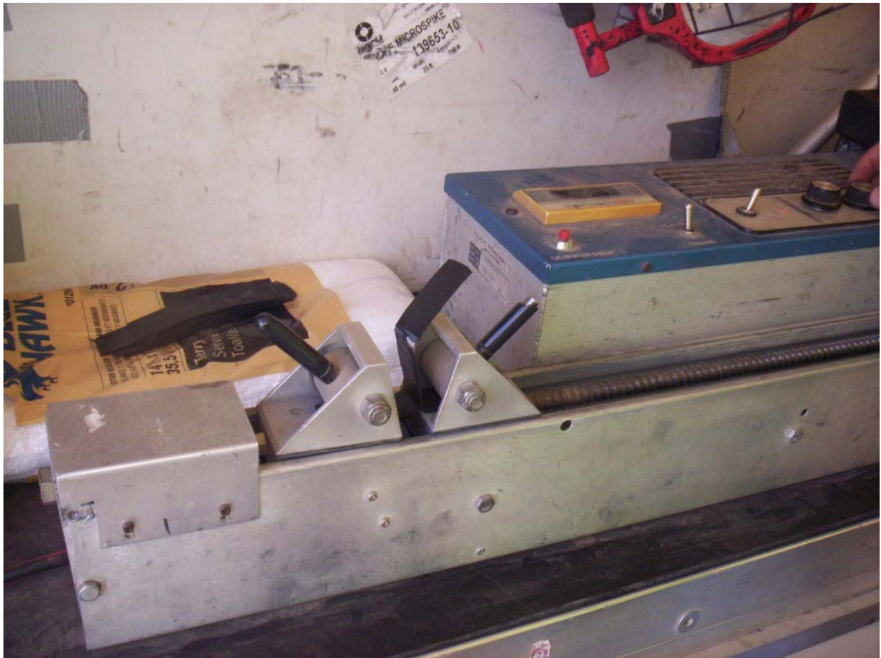
1590. On-site testing equipment for peel and shear tests
