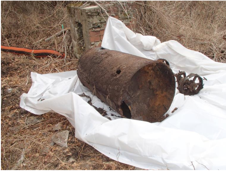
1) AOC-1: UST Area. View of UST and associated parts.
